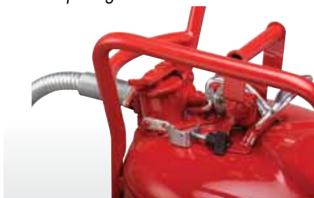
Type II D.O.T. Safety Can Two openings: top opening with lift lever for filling, and a second one with flexible metal hose attached for accurate, plug-free dispensing into smaller openings. Additional safety features include roll-bar construction and a fusible-link protected hold-down bracket for protection during over-the-road transport.
