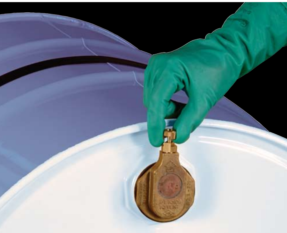
Above: Vacuum relief is manually controlled on a drum vent installed on a horizontally-positioned drum. Pressure relief is automatic.
